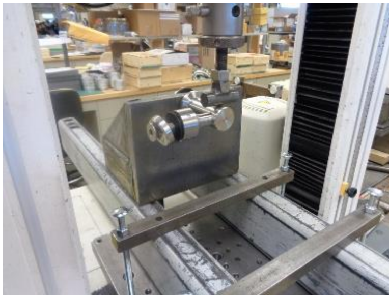
Photo No. 4 Typical Setup for Horizontal Shear Loading Classic VP Style Hook Fitting
