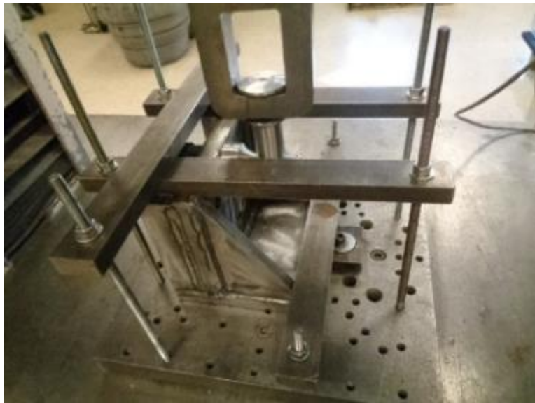
Photo No. 1 Typical Setup for Tension Loading Classic VP Style Hook Fitting
