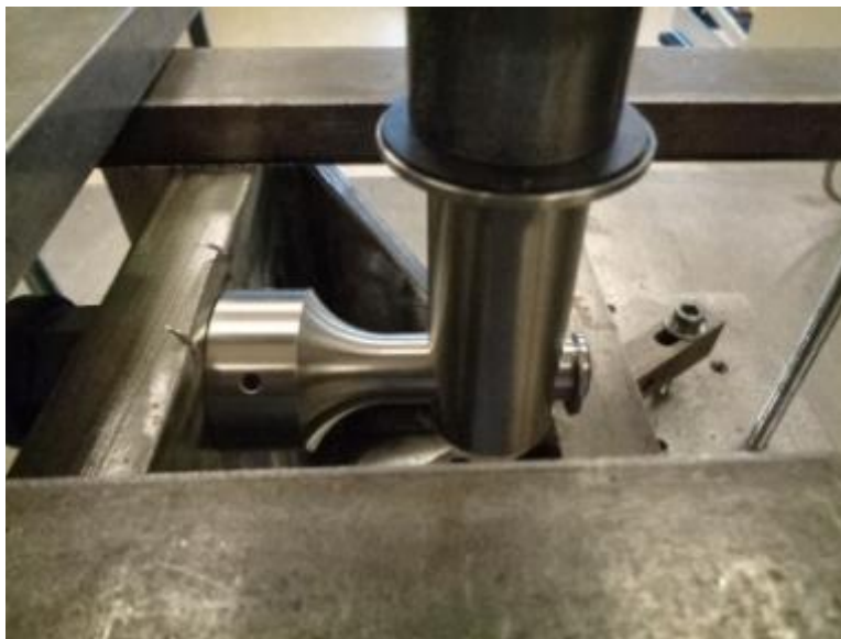
Photo No. 2 Typical Setup for Compression Loading Classic VP Style Hook Fitting
