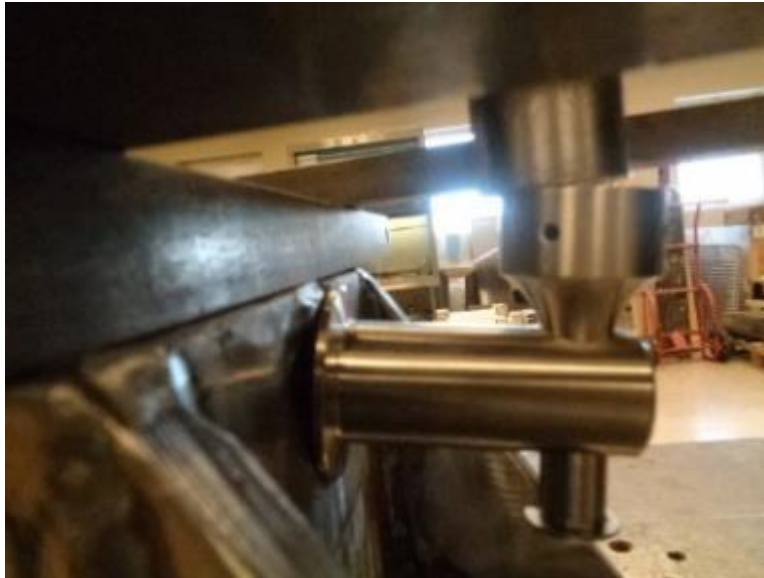
Photo No. 3 Typical Setup for Vertical Shear Loading Classic VP Style Hook Fitting
