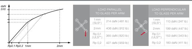
\*SLS: Serviceability Limit State - load at 1 mm deformation \*\*ULS - Ultimate Limit State: load at the elastic limit (Rp 0.1).
