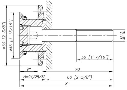
H= Swivel body corresponding to the thickness of the glass.  $V^*=$  glass thickness.
