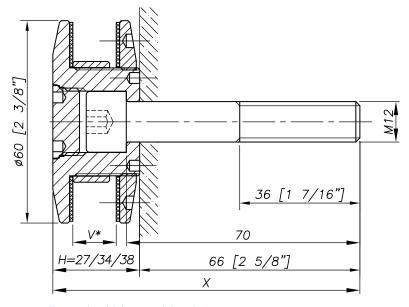
H= Swivel body corresponding to the thickness of the glass.  $V^*=$  glass thickness.
