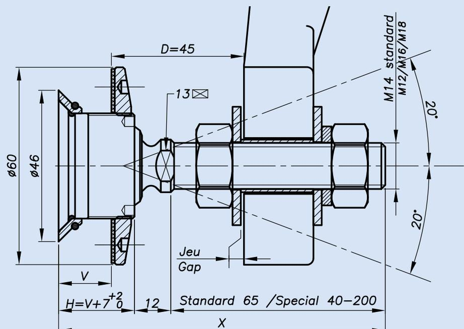
It is important to provide the following information with each request: the glass composition (ex.: 10 mm monolithic, 8.8.4 laminated, 8.8.2-12-10 insulating) / the length and diameter of the threaded axle if not standard dimensions (M14, 65 mm) / the reference of the spider to be used as support, or the thickness of an existing support for the delivery of the spacer.
