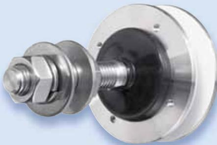
SADEV provides a protection from elements in the form of a silicone cover. Attention, this cover is not a simple option that you can add later. It is imperative to order a swivel fitting marked "SO" for this option since the swivel body is bigger and the glass nut is accordingly adapted.
